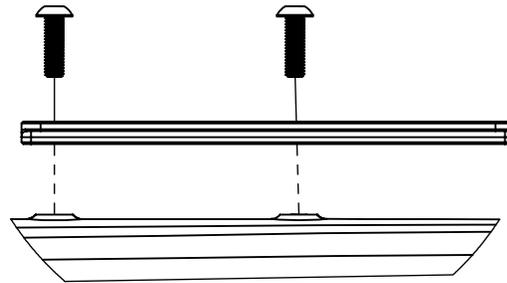
**STEP 3.** Mount accessories or bottle cages to the 2-slot base using "short" screws.
